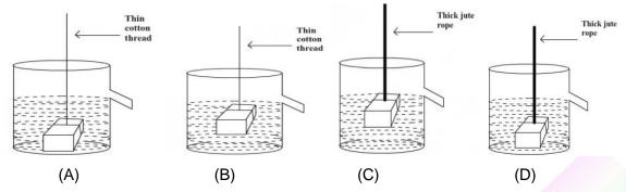
Ans: (b) The solid must be suspended in the centre of the overflow can and does not touches the bottom
