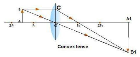
Let AB is an object placed between f1 and f2 of the convex lens. The image A1B1 is formed beyond 2F<sub>2</sub> and is real and inverted.
