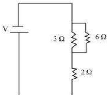
Here, 6 Ω and 3 Ω resistors are connected in parallel.
