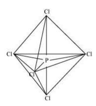
There are five P–Cl sigma bonds in PCl<sub>5</sub>. Three P–Cl bonds lie in one plane and make an angle of 120° with each other. These bonds are called equatorial bonds. The remaining two P–Cl bonds lie above and below the equatorial plane and make an angle of 90° with the plane. These bonds are called axial bonds. As the axial bond pairs suffer more repulsion from the equatorial bond pairs, axial bonds are slightly longer than equatorial bonds.
