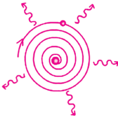
Fig. 07: The electron in the Rutherford's model is expected to spiral into the nucleus
