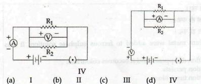
An ammeter and voltmeter are connected to calculate equivalent resistance when two resistors  $R_1$  and  $R_2$  are connected in parallel. Correct method of connection is :
