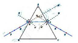
In case of a rectangular glass slab, emergent rays of light are always parallel to the direction of incident rays. Whereas when an incident light passes through a prism, it bends towards the base of the prism hence incident ray and emergent ray are not parallel to each other.
