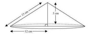
When right-angled  $\triangle$ ABC is revolved about its side 5 cm, a cone will be formed having radius (r) as 12 cm, height (h) as 5 cm, and slant height (l) as 13 cm.
