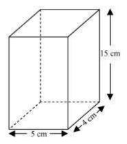
Length (I) of tin can = 5 cm Breadth (b) of tin can = 4 cm Height (h) of tin can = 15 cm
