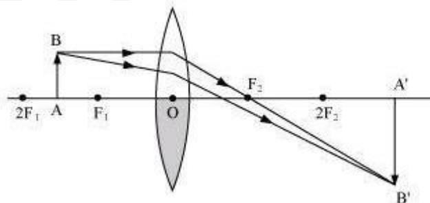
Question 24: An object 5 cm in length is held 25 cm away from a converging lens of focal length 10 cm. Draw the ray diagram and find the position, size and the nature of the image formed.
