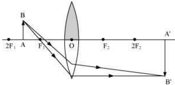
Case II When the lower half of the lens is covered
