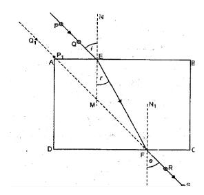
4. Now look through the glass slab form the other side and fix two pins (R and S), so that those pins and the image of the pins P and Q are in a straight line (when seen through the glass slab).
