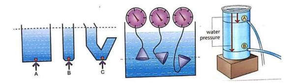
Ans: Figure 1: The pressure of water or any other liquid at a given depth does not depend upon the shape of the vessel containing the liquid or the amount of liquid in the vessel. It depends on the height of the column of liquid.
