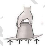
The air that presses upwards on the paper as shown in the illustration keeps the card paper fixed to the tumbler. This shows that air around us exerts pressure.
