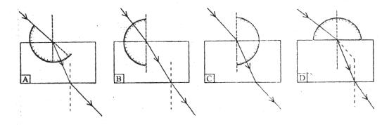
For measuring the angle of incidence, he must position the protector in the manner shown in figure.
